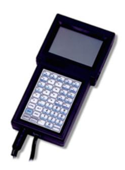
This document describes how to use the AnaCom Hand-Held Terminal (HHT) to monitor and control an AnaCom Transceiver (ODU) and AnaCom 1+1 Redundancy Systems. Hints on using other hand-held devices to monitor and control an ODU are provided as well.
