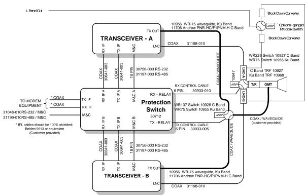
ANACOM 1 + 1 Redundancy Protection Switch Cabling Diagram
